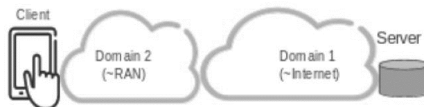
Figure 1 Reference scenario for the concept: the traffic between a Client and a Server crosses two domains with different characteristics (e.g., Internet and RAN, respectively)
