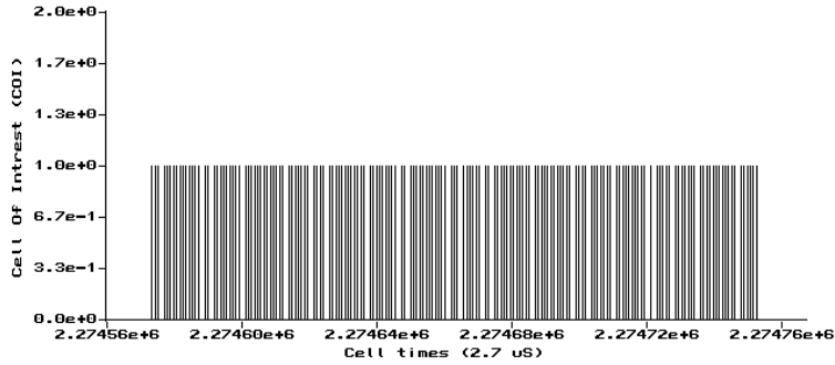
Fig. 16. VBR Video Cell Level (window length: 54.5 \mu s, average rate in the window: 144.7 Mbps)
