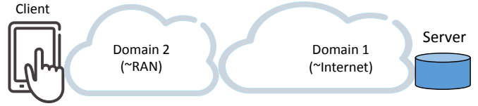
Fig. 1: Reference scenario for the concept: the traffic between a Client and a Server crosses two domains with different characteristics (e.g., Internet and RAN, respectively)
