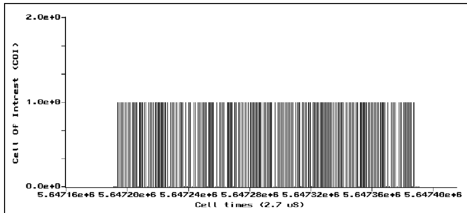
Figure 3.4: The cell arrival intensity of the PL25 sequence on cell level. Scale of the graph: 654 ms, mean rate in the graph: 133.4 Mbps, size of time window: 1 cell time.
